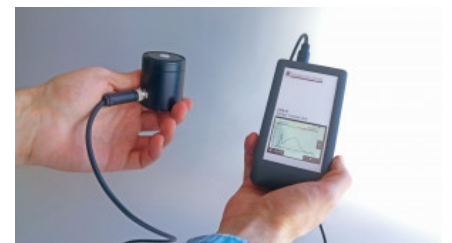
Use of CSS-45 as a handheld instrument by combining it with the control unit CSS-D
