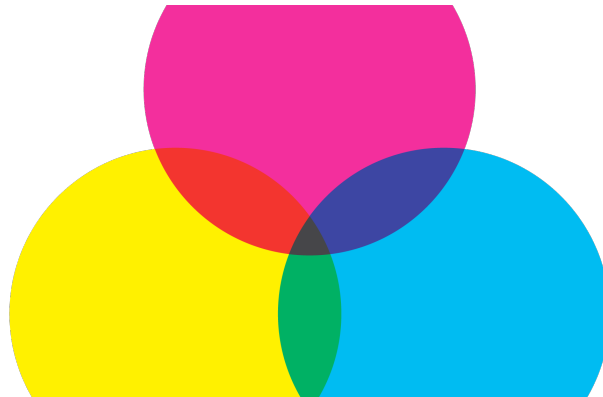
Fig. 4: Overlapping arrangement of yellow, cyan and magenta color filters on an overhead projector. In the overlapping regions, color subtraction results in green, red and blue light.
