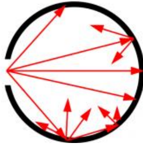
Fig. 1: Ideal multiple Lambertian reflections inside an integrating sphere
